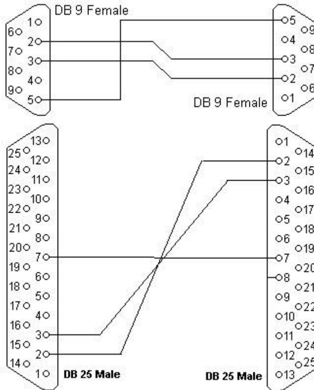
**Null modem with loop back handshaking**
