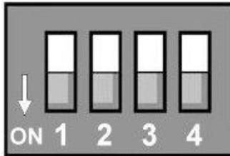
The switch is used to identify card number, default setting is card 15, and there are two methods to set the card number:
